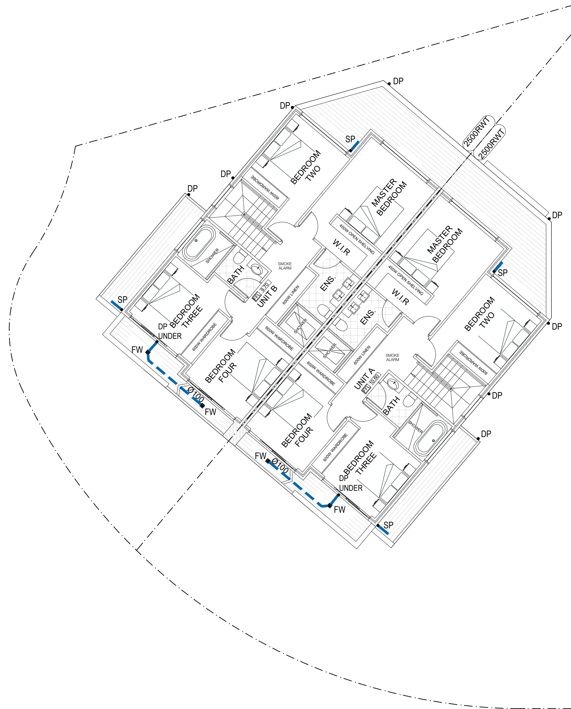
FIRST FLOOR STORMWATER DRAINAGE CONCEPT PLAN SCALE 1:100
